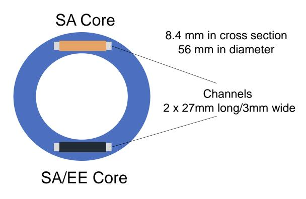
Total drug load = 103 mg SA/17.4 mg EE Daily release rate = 0.15 mg SA/0.013 mg EE
